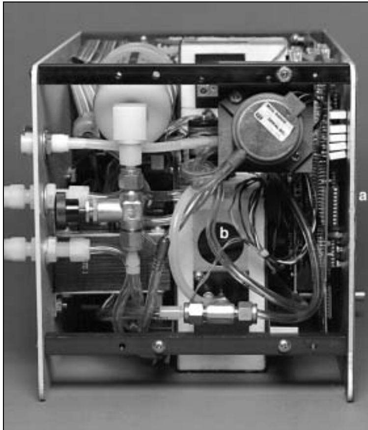
Figure 8-1 Locating the Filter Plug Inside the UCPC (a) Front Panel; (b) Filter Plug
