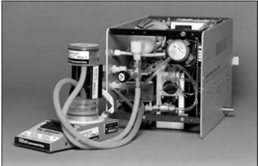
Figure 4-4 External Flowmeter in the Sheath-Air Line
