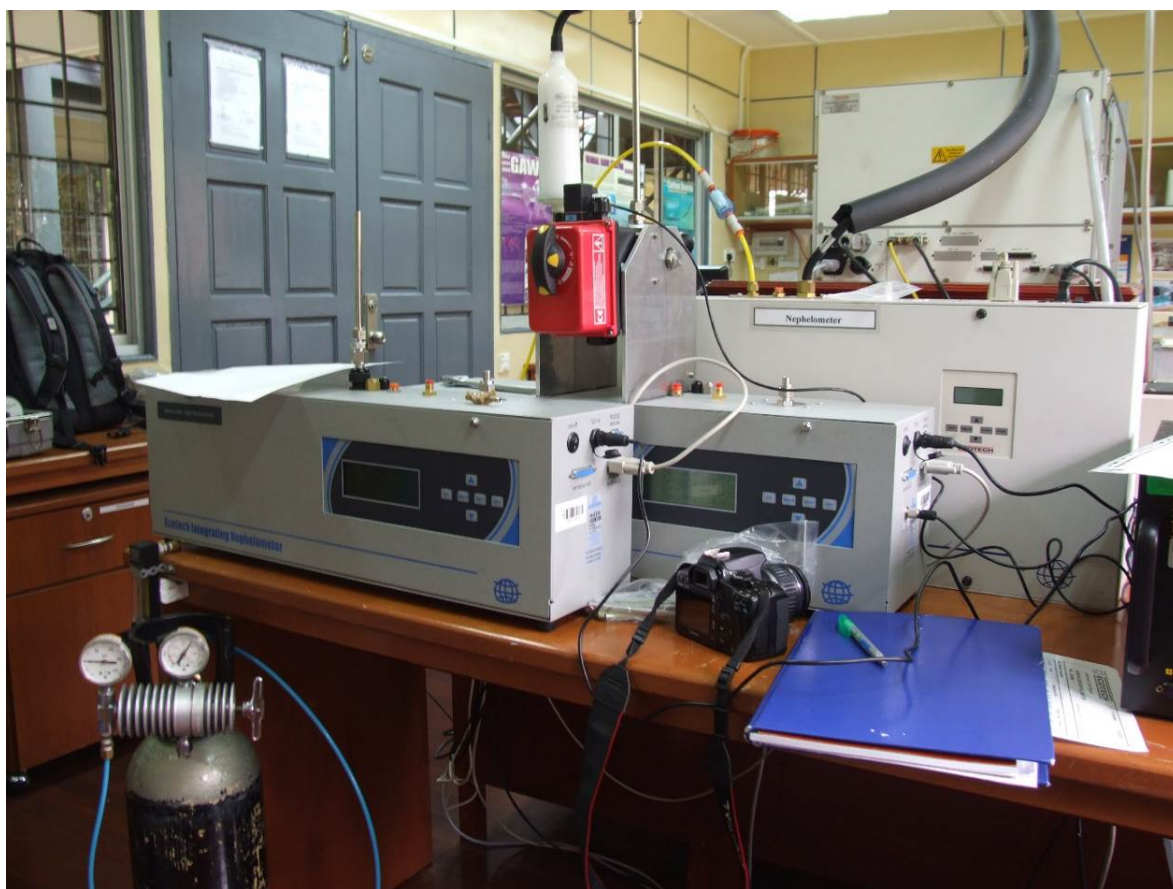
Figure 3: (from front to back) polar nephelometer Aurora 4000, new 3-wavelength nephelometer Aurora 3000 and old nephelometer.
