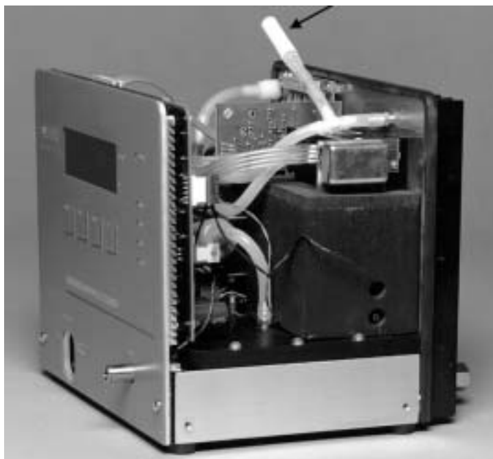
Figure 7-1 Inside View of the CPC-Purge Air Inlet and Filter
