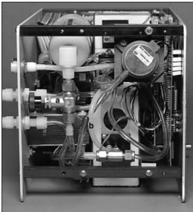
Figure 4-3 Location of Sheath Air Valve (a) and Bypass Variable Orifice (b)
