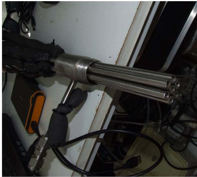
Figure 5: Flow splitter.
