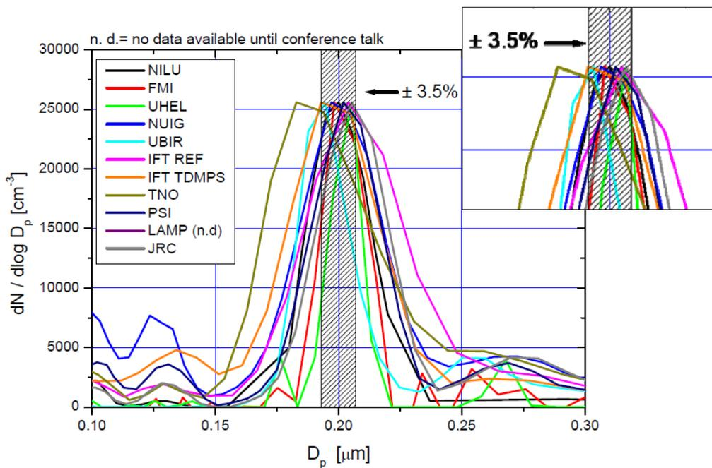
Figure 6: Raw number size distribution of 200 nm Latex measured during 2009 SMPS intercomparison workshop in Leipzig (black line, NILU).
