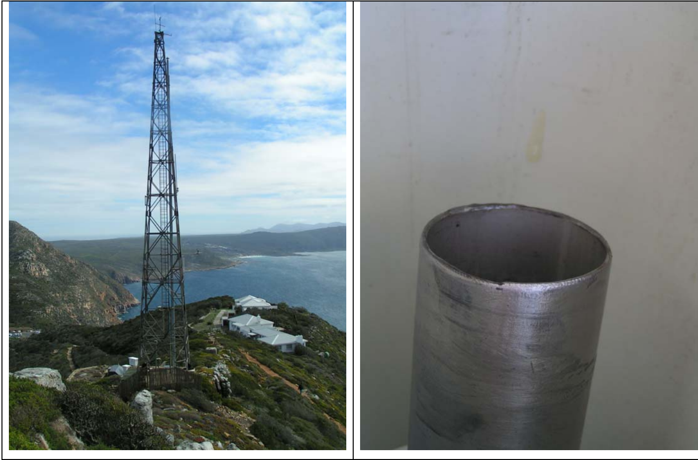
Fig. 1: Main aerosol inlet attached to the tower (left) and heated aerosol inlet (right)
